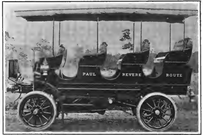
KNOX CONVERTIBLE STAGE WITH AIR-COOLED MOTOR.
